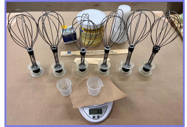
Overmolding using SLA printed 2 part molds
