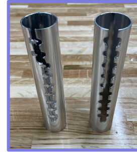
Poor machining of tube stock → Design Change
