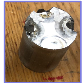
Welded thin aluminum was limiting → Design Change
