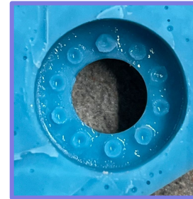
Wire holes were too small to mold → Design Change
