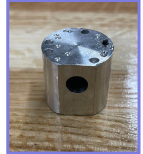
Wire holes were too small to machine → Design Change
