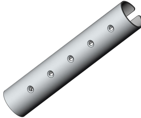
Handle - Turned on the Lathe & Milled
